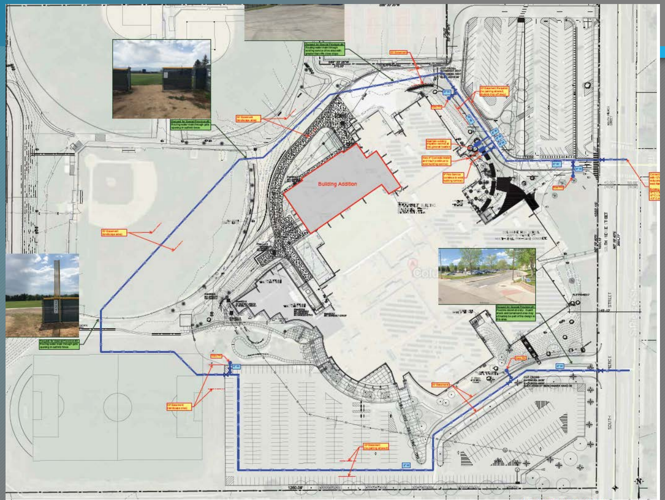
Original Water Pipe Configuration
