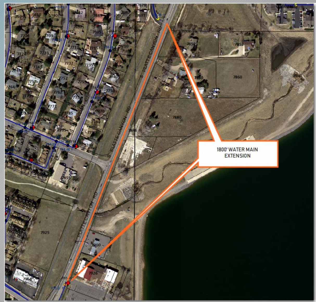
1800 Ft Water Main Extension
