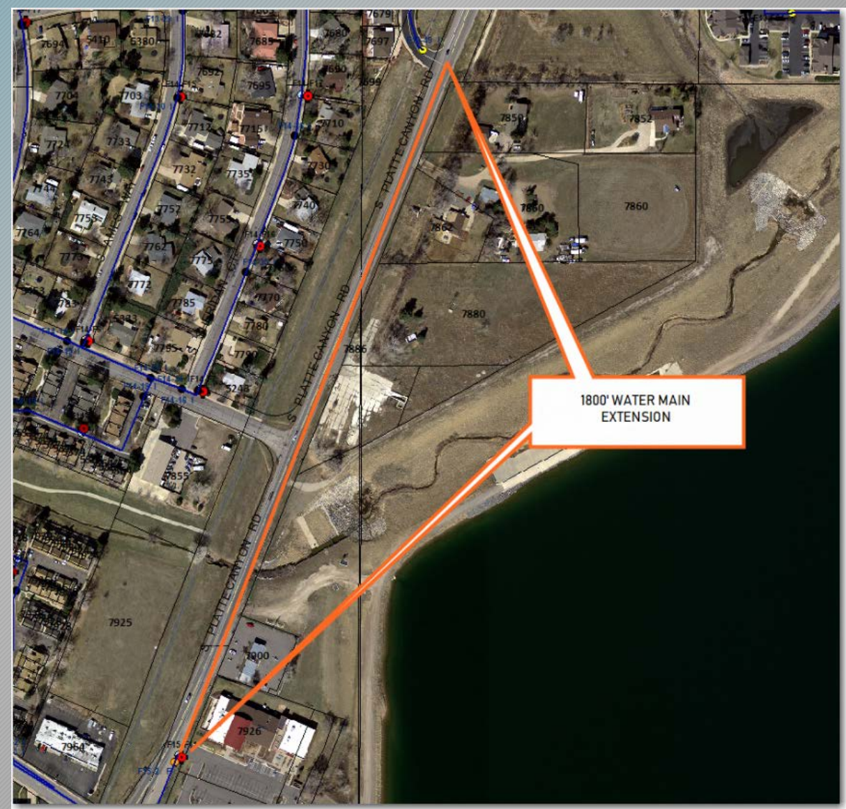
1800 Ft Water Main Extension
