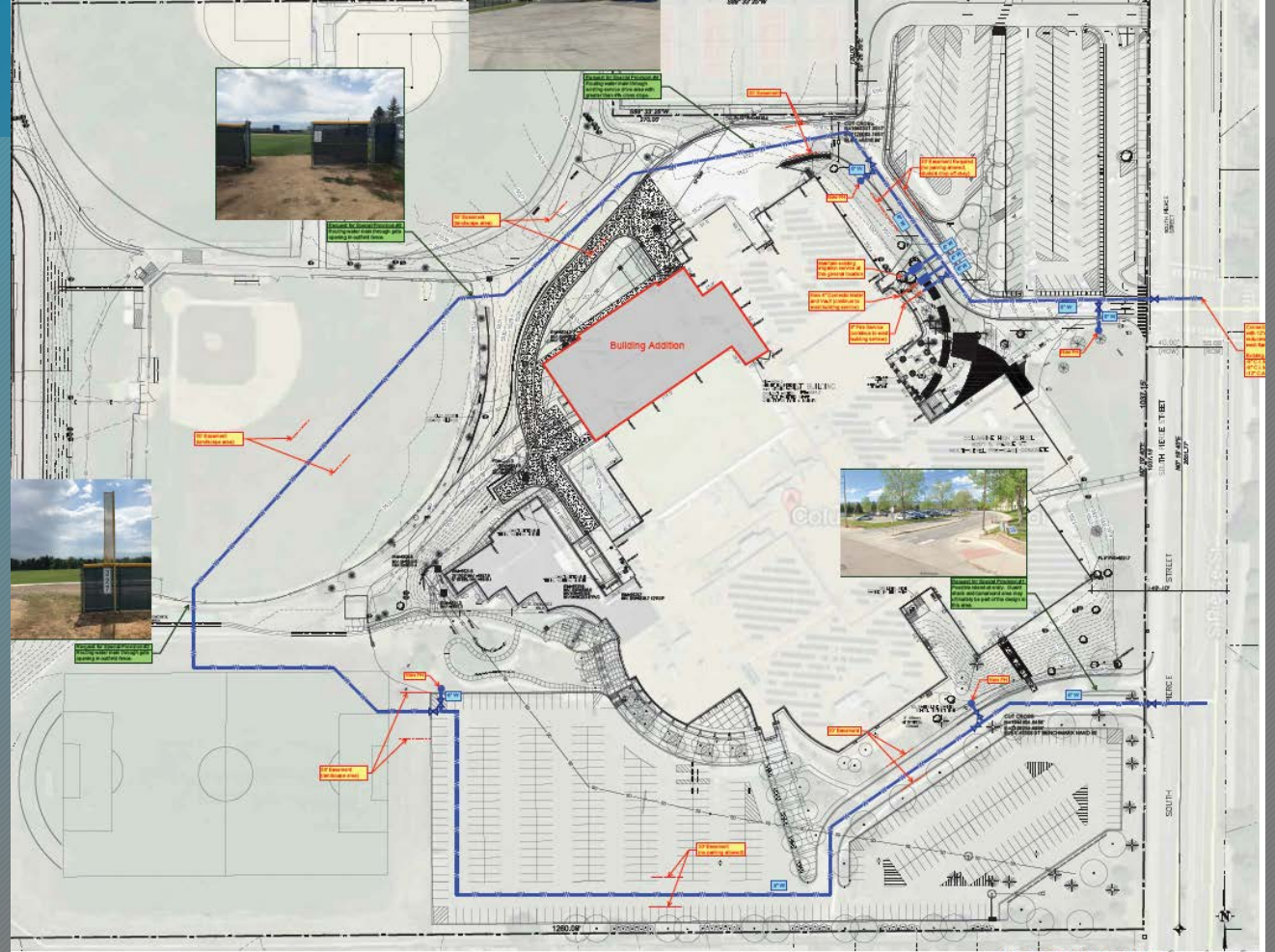
Original Water Pipe Configuration
