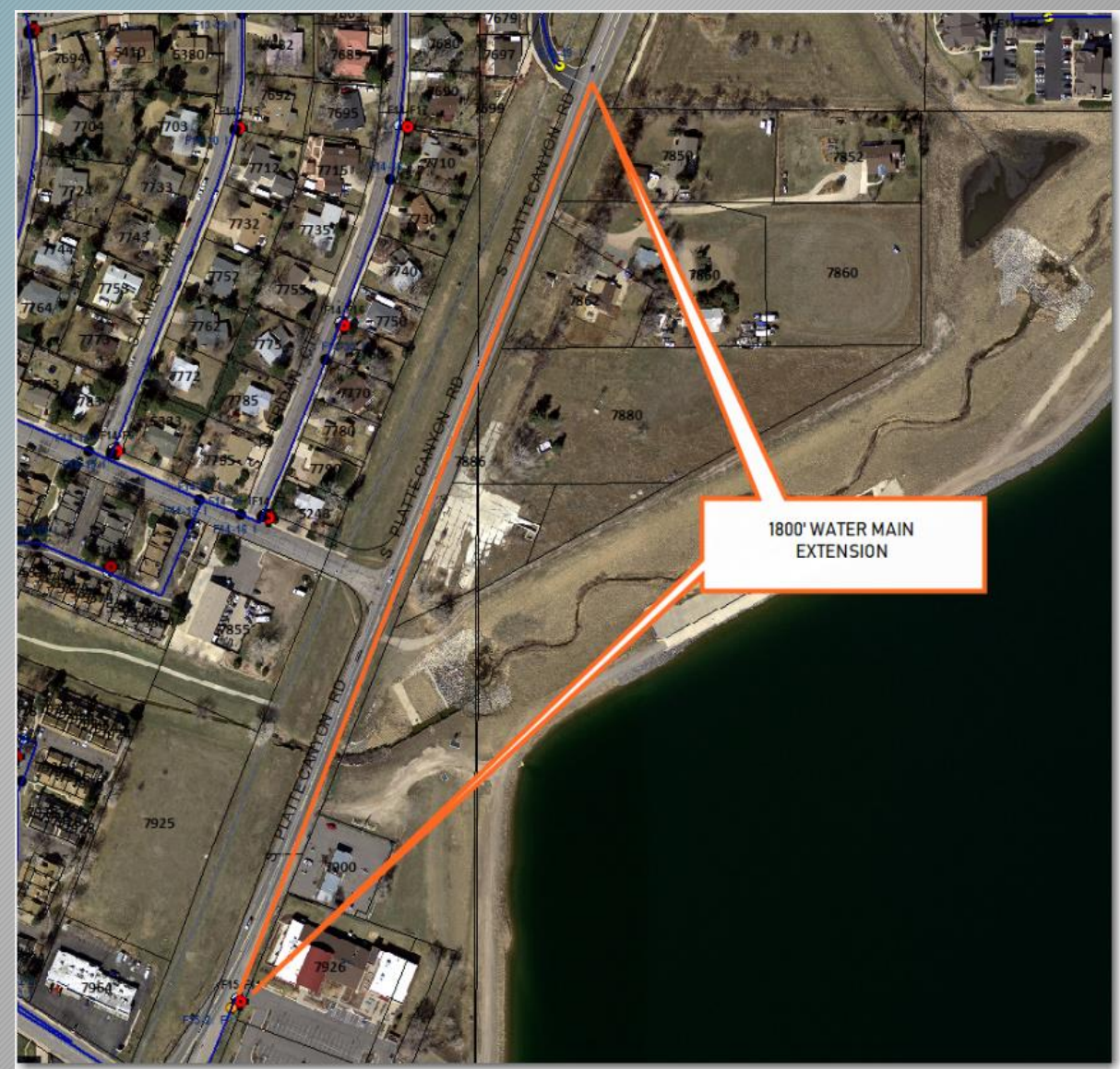
1800 Ft Water Main Extension
