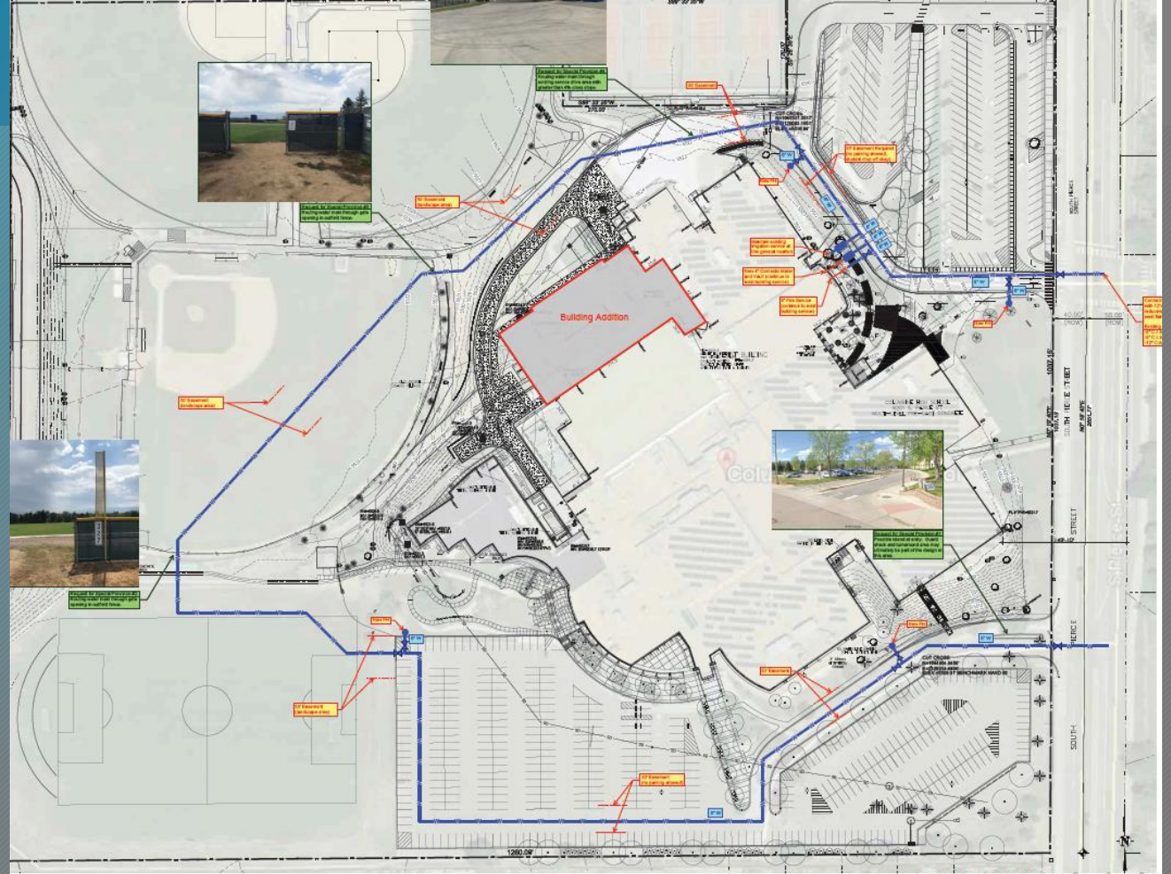
Original Water Pipe Configuration
