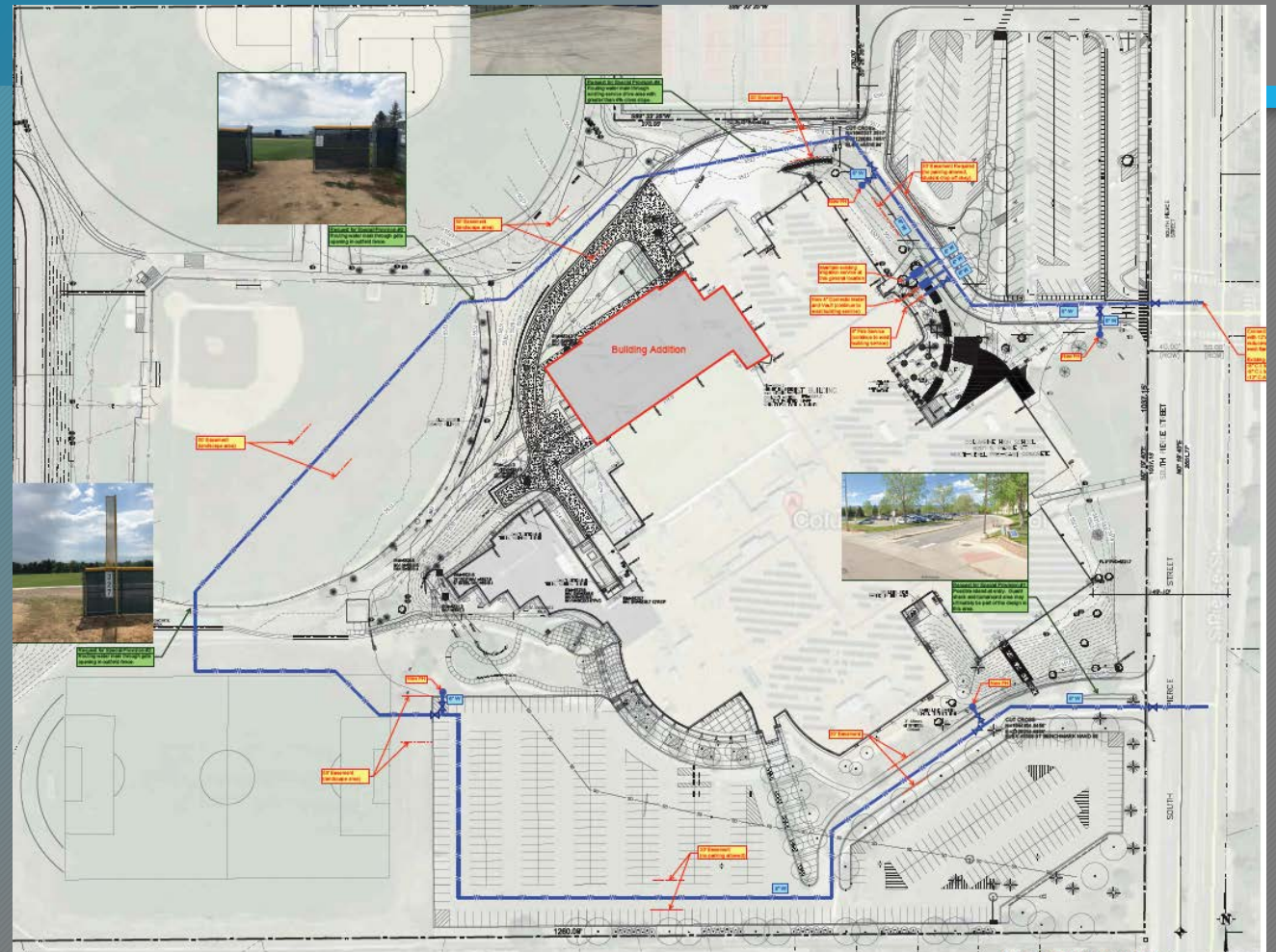
Original Water Pipe Configuration
