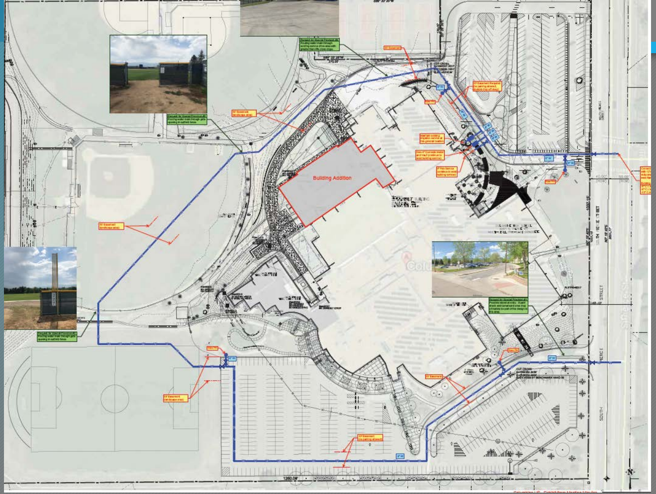
Original Water Pipe Configuration
