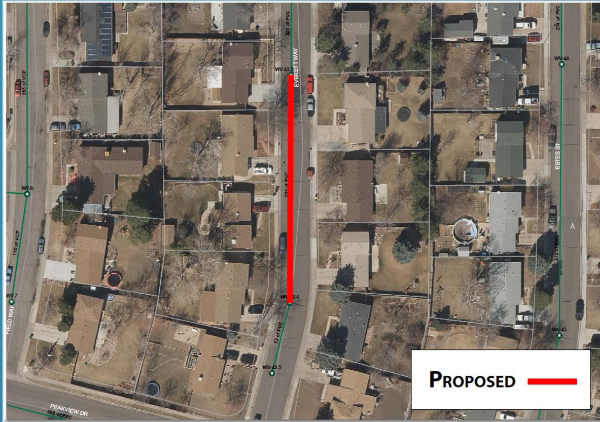
Everitt Way north of Peakview – Replace 227' of 8" Sewer main
